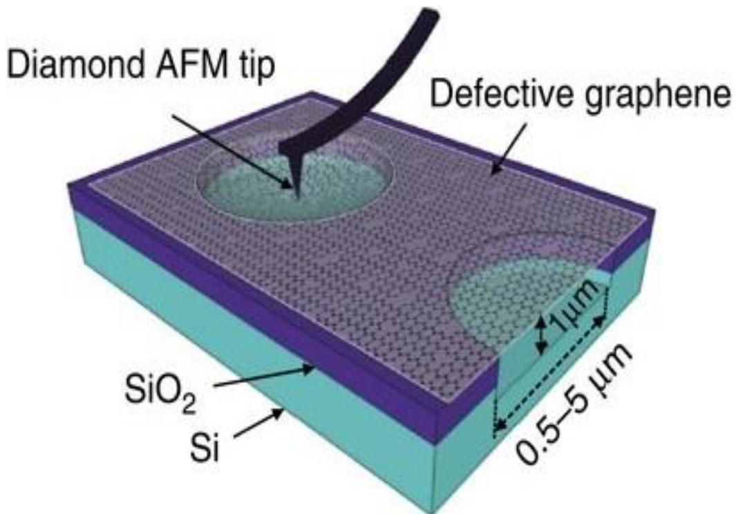
Figure 3. Graphene sheet testing by AFM tip
