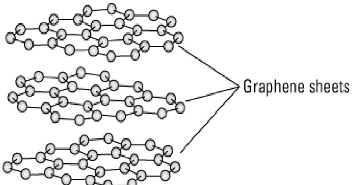
Figure 1. Structure of Graphene layers
