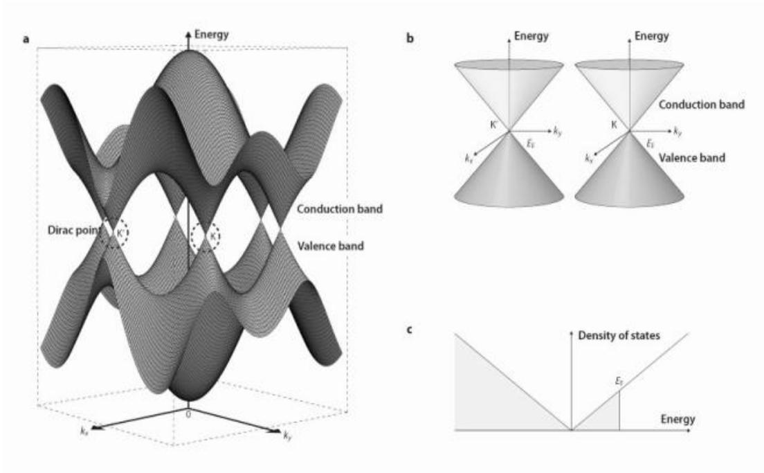
Figure 2. b) graphene  $\pi$ - and  $\pi^*$ -band structure over the complete Brillouin zone
