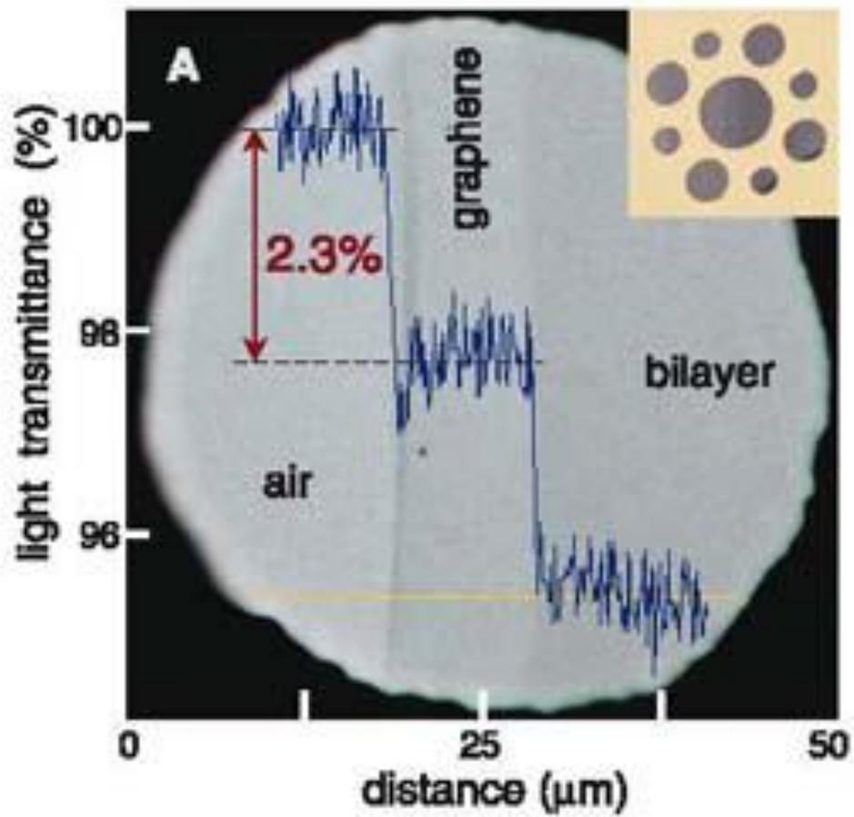
Figure 4. Transparency of Graphene Sheet
